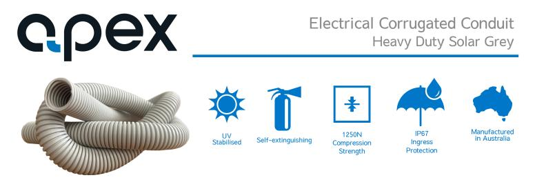
Australian manufactured heavy duty solar corrugated PVC conduit, designed for cable protection and management in domestic/commercial rooftop and static solar farm installations. Advanced UV stabilisation formulation suitable for long-life outdoor applications. Tested and compliant to AS/NZS2053.5:2001. Certified to Best Environmental Practice Standards BEP PVC.
